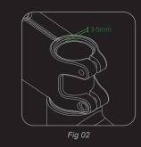
2.5: Install the top cap and compression bolt to the top of the Power Stem, as per the manufacturers specifications. This is typically until all the play is removed, yet the Power Stem can still smoothly rotate.
